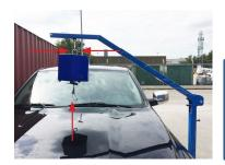
Making sure that the winch does not touch the vehicle, rotate the arm to check that when the winch is in the middle of the horizontal arm it is in the middle of the vehicle
