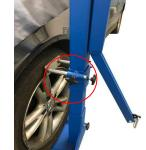
Raise the wheel support up in line with the tyre, loosen the side securing screws and extend the support until it touches the tyre, tighten screws back up.
