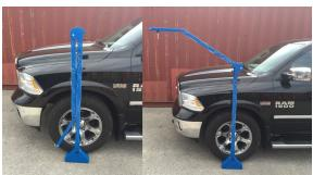
Insert the support arm and tighten the two screws in the wheel plate upright. Unfold the arm taking care not to touch the vehicle. Beware of any pinch points when unfolding the arm.
