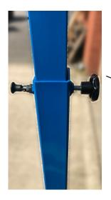
Once you have achieved your desired height using the lower vertical support ensure that the spring pin is correctly located and tighten the large security knobs to ensure the risk of a sudden drop is minimized.
