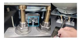
9. Re-install vacuum pump by placing in keyhole and sliding to the left. Use the wrench to tighten the 8mm bolts. Close machine front panel and lock latch; loadcell lock installation is now complete.
