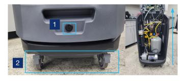
Remove vacuum pump using an 8mm socket to loosen the bolts underneath the baseplate, then sliding the pump the right to disengage. Gently place the pump on a raised surface at least 3 inches from to ground to avoid placing excessive tension on the internal hoses. It is important not to stretch or damage the vacuum hoses.
