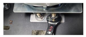
7. Engage loadcell lock, then attach sticker as shown
