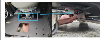
5. Place spacer bracket down, then insert the pins into the bracket sleeves. Level lock/push spacer bracket parallel with loadcell.
