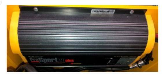
The above photograph shows the ProSport 43029 charger as installed in the SUPER PUSHER. The charger is located under the hinged lid of the battery compartment. In-line 15A fuses are fitted. Only use replacements of the same type and rating.
