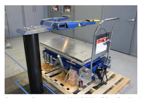
Step 1: To begin the process of removing your AGA Lift Table off the pallet, place the pallet under the arms of the lift in your shop.
