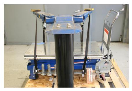
Step 5: Place straps over the arms of the lift. Adjust the ratchet straps to equal lengths.
