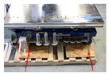
Step 3: Remove front and rear fixtures on both left and right side. Arrows shown in picture above indicate front and rear fixtures that need to be removed for removal process.
