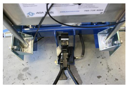
Step 7: Install handle with 4 supplied 10mm bolts and washers. Torque bolts to 40Nm (30lbs).
