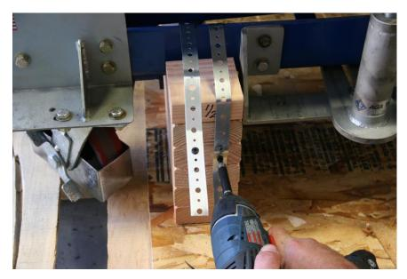
Step 2: Remove all screws secure metal straps on the outside only. Please note that there are 3 sections that are held down: one on the left, one on the right and one towards the front.
