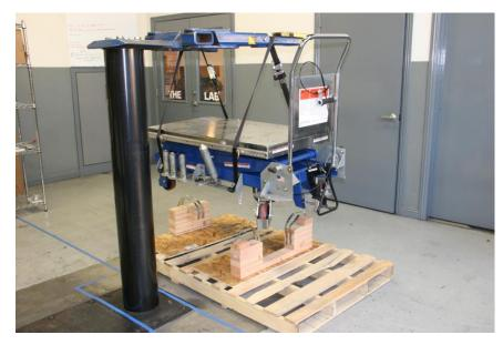
Step 6: Raise the lift till the Lift Table has completely detached itself from the pallet. Pull pallet out. Slowly lower lift until the Lift Table is on the ground. Remove ratchet straps and reinstall fixtures that were removed in step 3.
