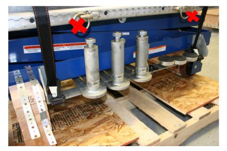
Step 4: Using the supplied ratchet straps, route them around the fixture rack as shown in picture.
