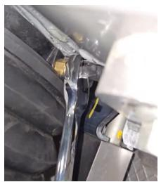
Reinstall voss fitting and use **TSN01525-300** socket to tighten fitting to air spring body. Torque fitting to spec using 16mm open ended "crowfoot"
