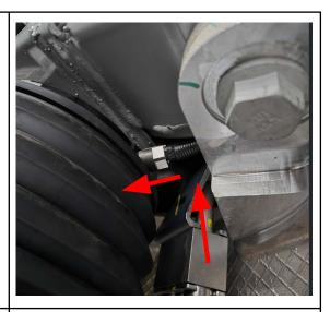
Use **16mm** open ended wrench to slowly loosen the fitting until free from the air spring body
