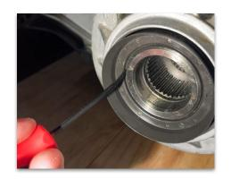
Pry on the seal gently till the seal starts to move. Move the tool into other positions around the circumference in order to evenly work the seal out.
