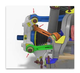
Use a 19mm socket and ratchet to drive the FORCING SCREW inward, pushing the axle out of the hub.
