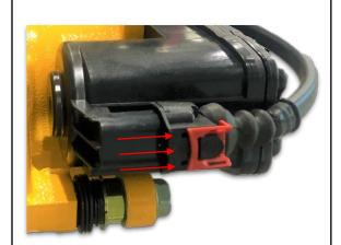
To disconnect vehicle harness, depress the release tab while pulling connector away from parking brake.
