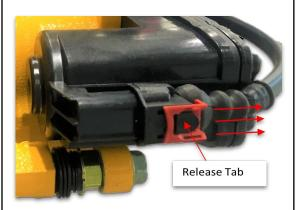
Install the EPB Adapter Harness to EPB, an audible click indicates a fully seated connector.
