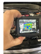
Picture in Picture setup showing the hot coolant flow in the system
