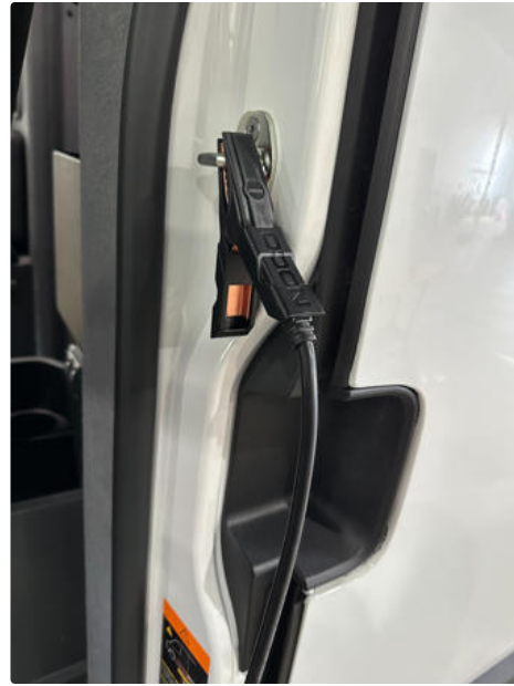
Negative Clamp Attached to Door Striker
