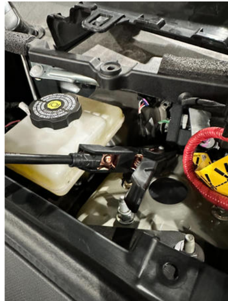
Negative Clamp Attached to Strut Mount
