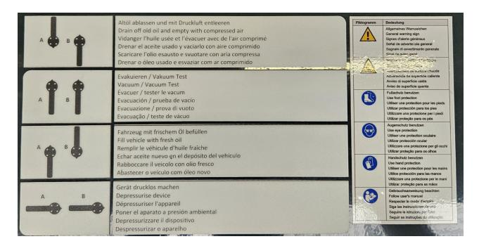
Guide to lever positions that will be used during the Evacuation/ Fill process with the EBS-100. It is located on top of the unit (Top Left)
