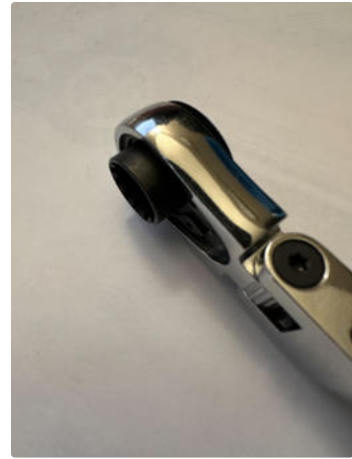
Step side of the 13mm ratcheting wrench, Allows to contact the fastener in locations where there is a surrounding lip
