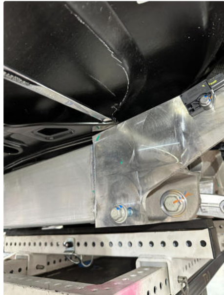
Passenger side tool access with subframe partially lowered (R1T shown, R1S is similar)
