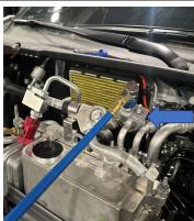
Connect the LP (BLUE) line from the AC machine to the BLUE LP R1234yf connector on the Mastercool Sight glass unit. Open the valve on the LP BLUE hose from the AC machine by turning the top of the coupler to compress against the Shrader.
