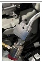
2 Connect the Low side (BLUE) on the AC flush kit to TSN01500-204-A GEN 2 COMPRESSOR LS (LOW SIDE) FLUSH ADAPTER on the vehicle.
