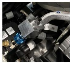
You will connect the LP (BLUE) line from the AC machine to the BLUE LP R1234yf connector on the Mastercool Sight glass unit. You will need to open the valve on the LP BLUE hose from the AC machine by turning the top of the coupler to compress against the Shrader
