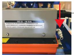
AIR SUPPLY: Pressure must be between 110 - 150 psi (7.5 - 10.5 bar). Air must be supplied to raise and lower the table.
